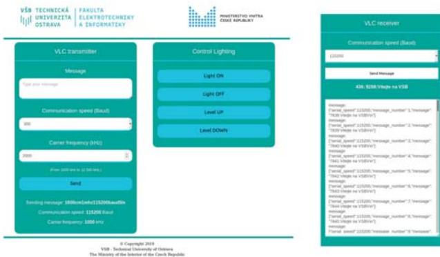
Fig. 4. The web visualization to control and set baud rates and data for the modulator with Bias-Tee.
