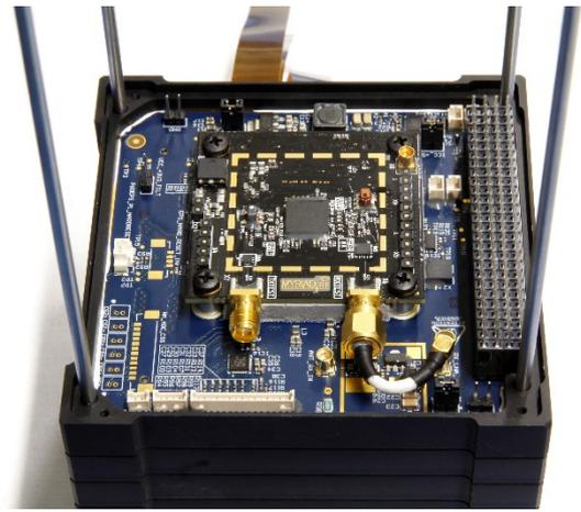
Fig. 8. The first-generation SDR motherboard with the MyriadRF daughterboard assembled into the flight housing frame.
