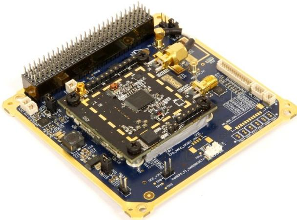
Fig. 7. The first-generation SDR motherboard with the MyriadRF daughter board. A thermal gap filler material is inserted between the two PCBs and special edge contacts are used to improve the thermal design.
